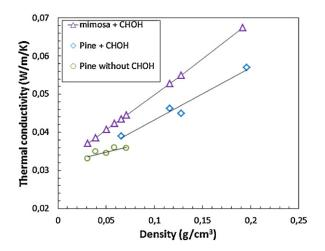
Fig. 4. Thermal conductivity as a function of foam density for pine tannin foams with and without formaldehyde and mimosa tannin foams with formaldehyde (control).
