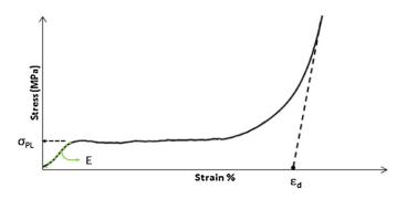
**Fig. 2.** Schematic example of stress-strain curve of compression in the growing direction of the foam (*z*-axis) for pine tannin-based foams with formaldehyde (density =  $0.065 \text{ g cm}^{-3}$ ).
