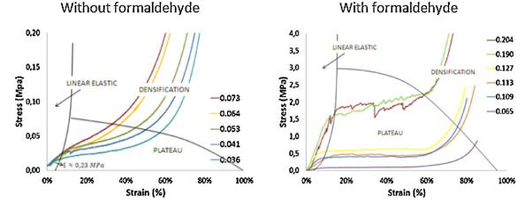
Fig. 5. Stress-strain curves of pine tannin-based foams (a) with formaldehyde, and (b) without formaldehyde (blowing agent = DE). Foam densities in g cm<sup>-3</sup> are listed in the figure.
