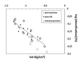
**Fig. 8.** Densification as a function of foam density for pine and mimosa tannin foams with formaldehyde and using DE and pentane as blowing agents.
