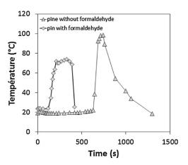
**Fig. 3.** Temperature as a function of time within a pine tannin-based foam mixture during foaming (DE = 3 g).
