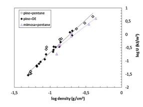
**Fig. 9.** Energy absorbed under compression by tannin foams as a function of foam density.
