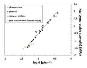
**Fig. 7.** Compression strength as a function of density for pine and mimosa tannin foams (blowing agent either DE or pentane).
